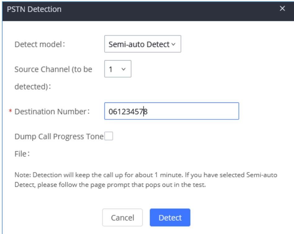
Figure 17: UCM6XXX PSTN Detection: Semi-Auto Detect
