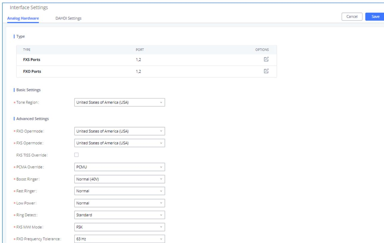
The screenshot shows the 'Interface Settings' window with the 'Analog Hardware' tab selected. It contains a table for port types and a list of settings for FXO ports.
