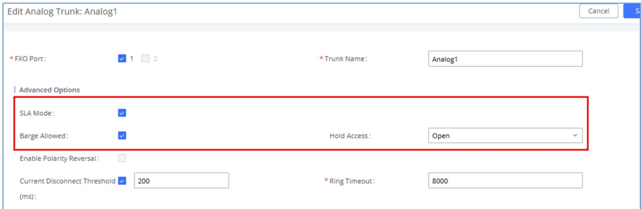
The screenshot shows the configuration interface for an analog trunk named 'Analog1'. The 'FXO Port' is set to 1. The 'Trunk Name' is 'Analog1'. In the 'Advanced Options' section, 'SLA Mode' is checked, 'Barge Allowed' is checked, and 'Hold Access' is set to 'Open'. Other settings include 'Enable Polarity Reversal' (unchecked), 'Current Disconnect Threshold' (200 ms), and 'Ring Timeout' (8000 ms).
