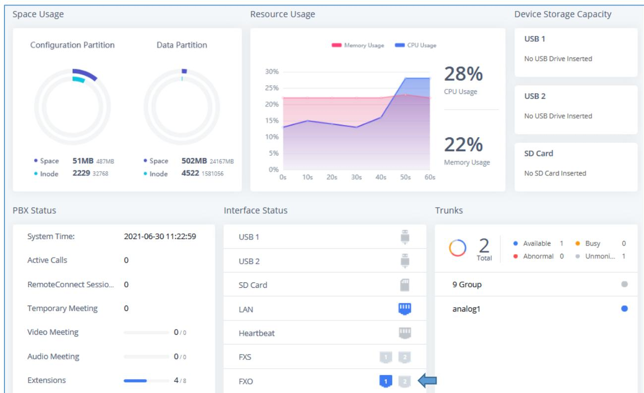
Figure 2: FXO Port Connected but not Configured
