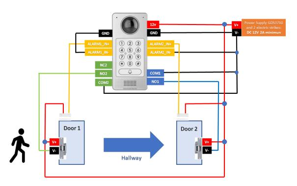
Figure 2: One-Way Interlocking Mode Diagram Example
