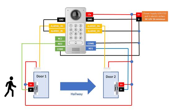
Figure 1: One-Way Interlocking Mode
