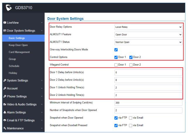
Figure 3: One-Way Interlocking Mode - GDS3710 Configuration 1
