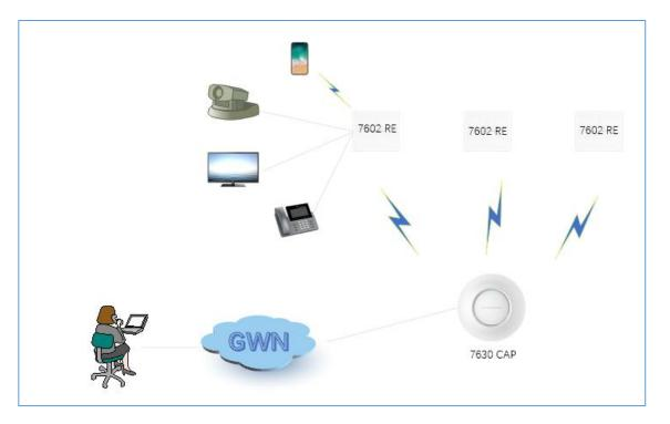
Figure 1: Wireless access layer network topology
