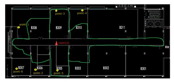
Figure 4: CAP Direct wall-trough coverage
