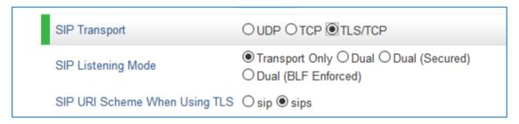
Figure 6 : Configure TLS as SIP Transport
