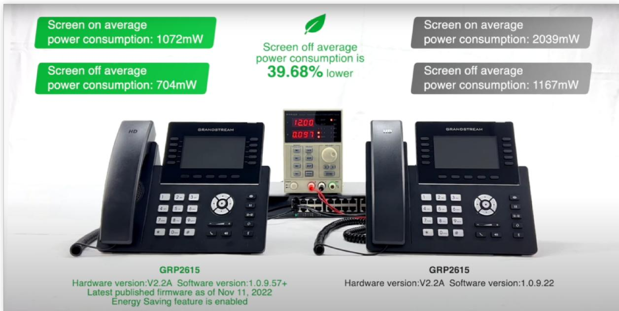
Alternatively, the illustration below compares the power consumption of Grandstream carrier-grade IP phones with those of competitors.
