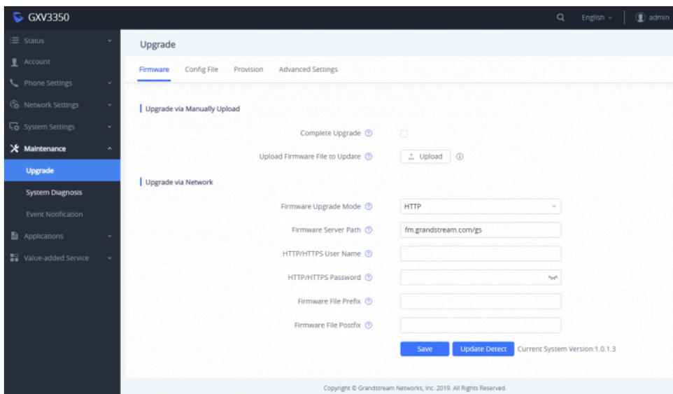
Figure 11: GXV3350 Upgrade Configuration via Web GUI
