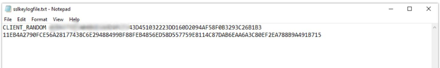
The extracted key gives you the possibility to decrypt the secured communication between the HT8xx and the SIP server.
