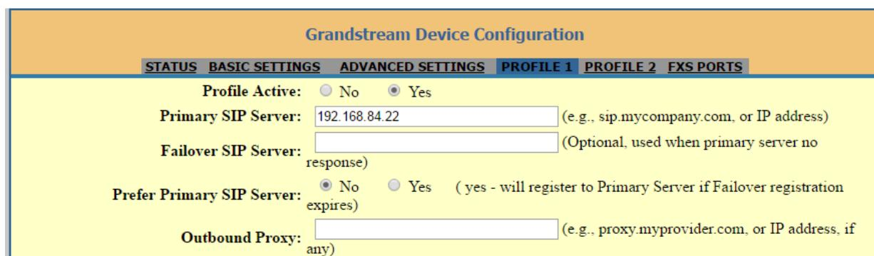
The screenshot shows the 'Grandstream Device Configuration' web interface. At the top, there are tabs for 'STATUS', 'BASIC SETTINGS', 'ADVANCED SETTINGS', 'PROFILE 1', 'PROFILE 2', and 'FXS PORTS'. The 'PROFILE 1' tab is selected. The settings for Profile 1 are as follows:
