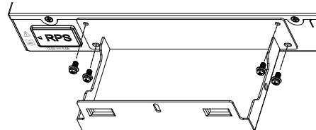
**Step 3:** Place the RPS horizontally into the bracket. Please ensure that the power cord is located on the side of the RPS silicone plug.
