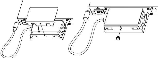
**Step 5:** Lift the RPS silicone plug from the arrow side and rotate it 90° clockwise to see the power hole, next connect the RPS to the switch, then connect the AC power cord to the RPS, finally complete the connection between the power cord and the power supply system.
