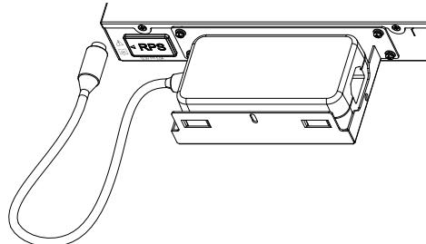
**Step 4:** Lower the bracket cover and ensure that the screw holes are aligned. Then, use the fixed screw (M3\*6) to lock the RPS inside the bracket.
