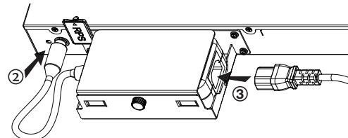
**Step 6:** To prevent accidental disconnection of the RPS, it's recommended to use a power cord anti-trip for installation. Place the smooth side of the fixed strap towards the power cord and connect it to the anti-trap hole below the power cord.
