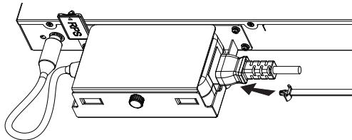
**Step 7:** Slide the protective rope over the fixed strap until the end of the power cord, then smoothly wrap the strap around the power cord and lock it tightly.
